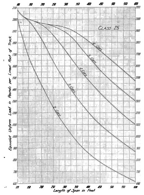
Fig. 6k. Equivalent Uniform Live Loads for Truss Spans with Class 25 Electric Railway Loading.
