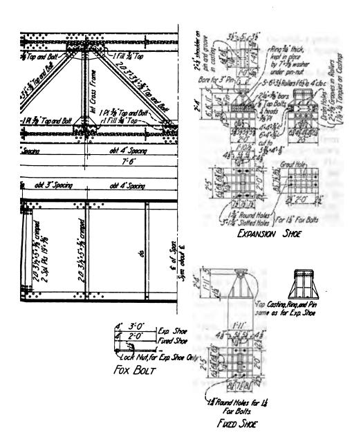
Span with Flanges Composed of Two Angles and Cover-plates.
