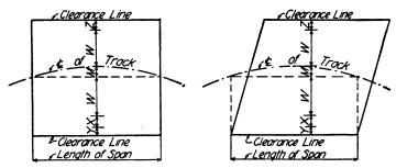
Fig. 8c. Clearance Diagram for Square, Through Bridges on Curves.
