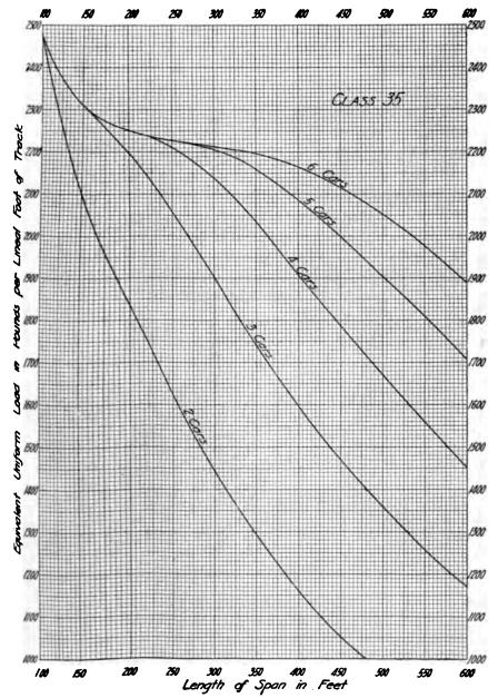
'16. 6m. Equivalent Uniform Live Loads for Truss Spans with Class 35 Electric Railway Loading.
