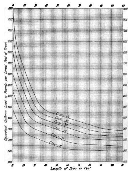
Fig. 6h. Equivalent Uniform Live Loads for Plate-girder Spans of Electric Railway Bridges.
