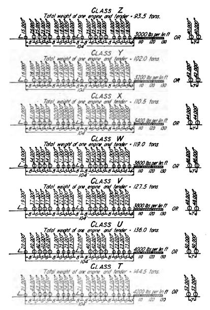
716. 6a. The Compromise Standard System of Live Loads for Railway Bridges.
