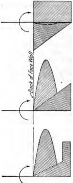
Fig. 43g. Loads on Base Slab of Counterforted Retaining Wall.
