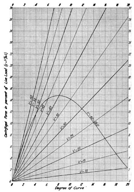
Fig. 8b. Centrifugal Force for Tracks on Curves.
