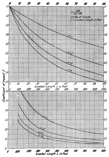
Fig. 7c. Coefficients of Impact for Railway Bridges.
