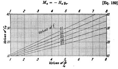
Fig. 37gg. Values of Temperature Stress Coefficient Cs.
