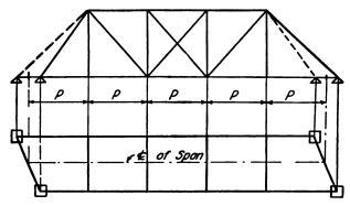
Fig. 224. Arrangement of Trusses for a Skew Span in which the Skew is Too Short for an Economical Panel Length.
