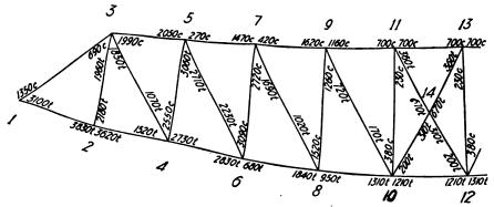
Fig. 11j. Secondary-stress Diagram of a 296-foot, Single-track-railway, Riveted, Parker-truss Span.
