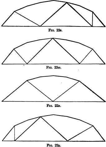
Systems of Lattice Truss with Polygonal Top Chord.
