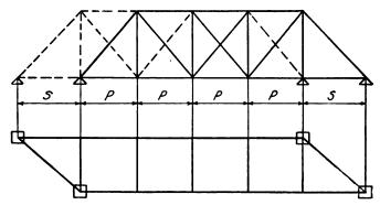
Fig. 22mm. Arrangement of Trusses for a Skew Span in which the Skew is Too Long for an Economical Panel Length.
