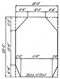
Fig. 22ii. Clearance Diagram for Through Bridges on Tangent.
