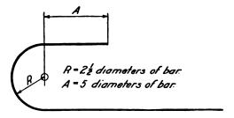
Fig. 37ww. Detail of Hook for Reinforcing Bar.
