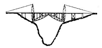
Fig. 26b. Three-hinged, Lenticular, Braced-rib Arch.
