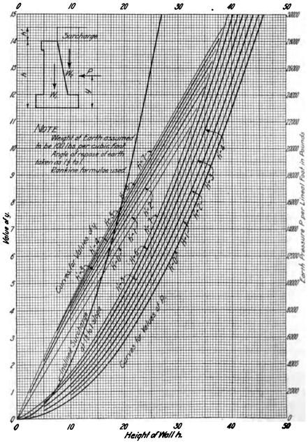
Fig. 43c. Earth Pressures for Retaining Walls.
