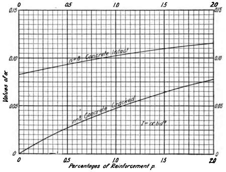
Fig. 37s. Moments of Inertia of Rectangular Beams.
