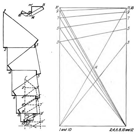
Fig. 12e. Williot-Mohr Diagram for a 296-foot, Single-track-railway, Riveted, Parker-truss Span.
