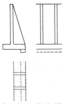
Fig. 43e. Counterforted Retaining Wall.
