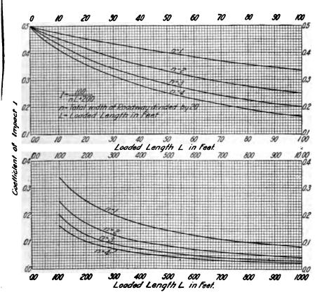
Fig. 7e. Coefficients of Impact for Highway Bridges.
