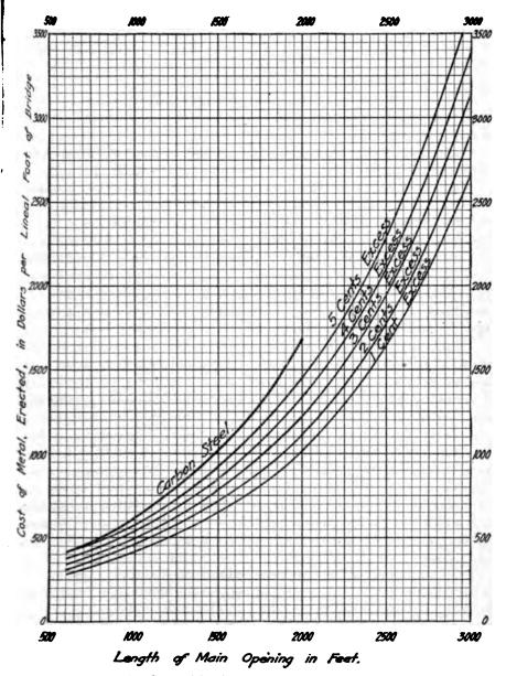
Fig. 40. Comparative Costs of Double-track, Cantilever, Railway Bridges of Carbon Steel and Mixed Alloy and Carbon Steels for  $E=80{,}000~\rm{lbs}$ .
