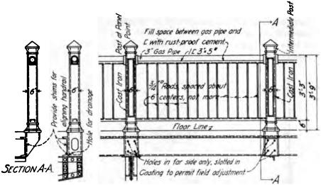
Fig. 19l. Bar-type Handrail.
