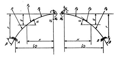
Fig. 37hh. Sketch of Arch Rib.
