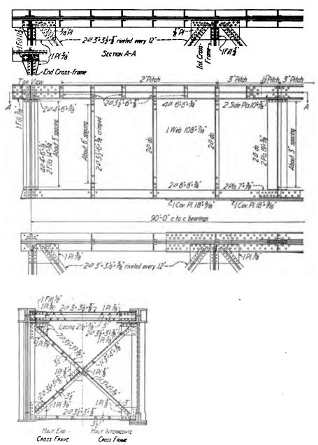
Fig. 21w. Details of a Single-track-railway, Deck, Plate-girder Span with a Four-angle Top Flange Section.
