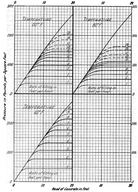
Fig. 37vv. Pressure of Wet Concrete on Forms.
