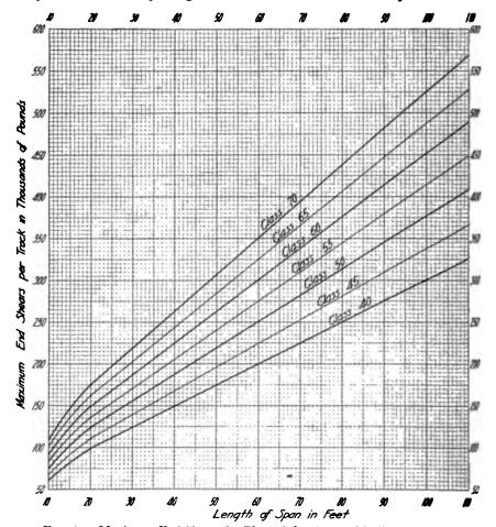
Fig. 6c. Maximum End Shears for Plate-girder Spans of Railway Bridges.
