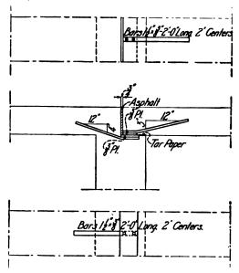
Fig. 37pp. Expansion Plates for Slabs.
