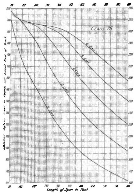
46. 6k. Equivalent Uniform Live Loads for Truss Spans with Class 25 Electric Railway Loading.
