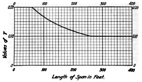
Fig. 9e. Traction Loads for Railway Bridges.
