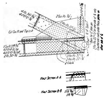
Fig. 26p. Crown Hinge for the Arch Span of the Canadian Northern Pacific Railway
