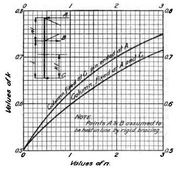
Fig. 16d. Points of Contraffexure in Braced Columns.
