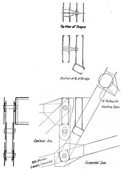
Fig. 25hh. Detail of Connection between Suspended Span and Cantilever Arm for the Transmission of Wind Loads.
