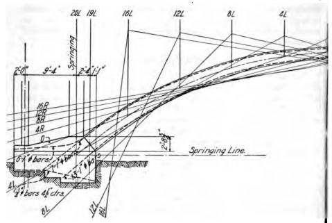
Fig. 37kk. Reaction Lines for an Arch Abutment.
