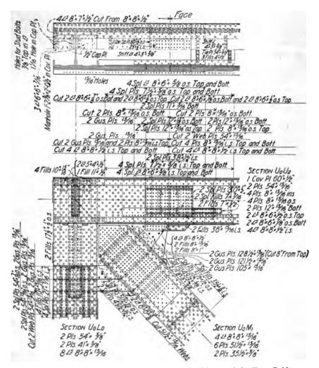
Fig. 22qqq. Top Chord Joint  $U_o$  of the 423-foot Fixed Spans of the Fratt Bridge over the Missouri River at Kansas City, Mo.
