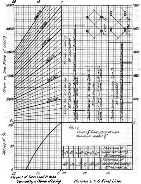
Fig. 16c. Diagram for Designing Lacing.
