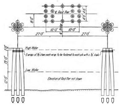
Fig. 36b. Fender Piles for the Lulu Island Bridge in British Columbia.
