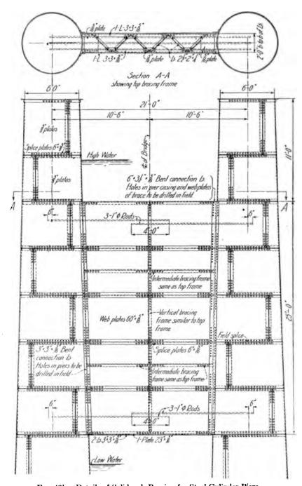
Fig. 43b. Details of Solid-web Bracing for Steel Cylinder Piers.
