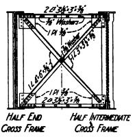
Fig. 21v. Details of a Single-track-railway, Deck, Plate
