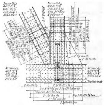
Fig. 22ppp. Bottom Chord Joint L<sub>2</sub> of the 287-foot Span of the O.-W. R. R. & N. Company's Bridge over the Willamette River at Portland, Ore.
