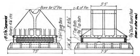
Fig. 22vvv. Shoe for the 423-foot Fixed Spans of the Fratt Bridge over the Missouri River at Kansas City, Mo.
