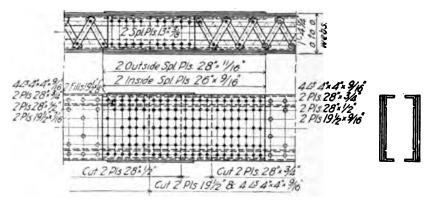
Fig. 22ggg. Tension Lap-splice in Panel LaL of the 271-foot Spans of the Great Northern Railway Co.'s Bridge over the Yellowstone River.
