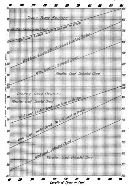
Fig. 9b. Wind Loads and Vibration Loads for Railway Bridges.
