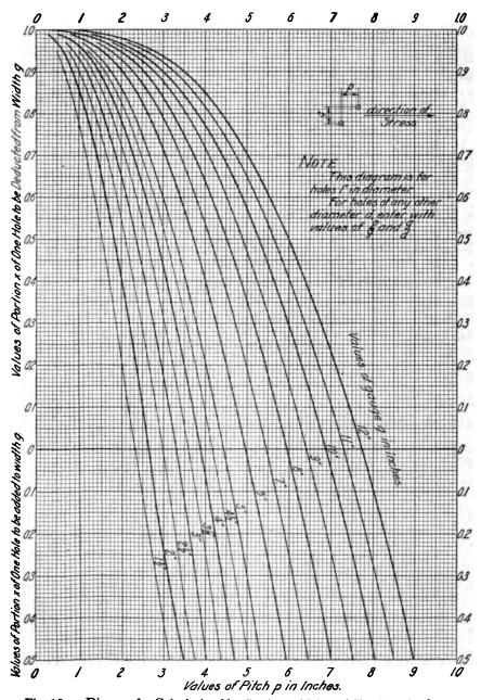
Fig. 16e. Diagram for Calculating Net Sections of Riveted Tension Members.
