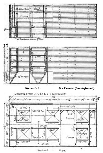
Fig. 40b. Open-dredging Caisson and Cofferdam for the O.-W. R. R. & N. Co.'s Bridge over the Willamette River at Portland, Ore.
