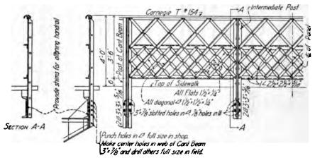
Fig. 19k. Lattice-type Handrail.
