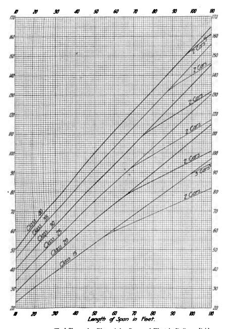
. 69. Maximum End Shears for Plate-girder Spans of Electric Railway Bridges.
