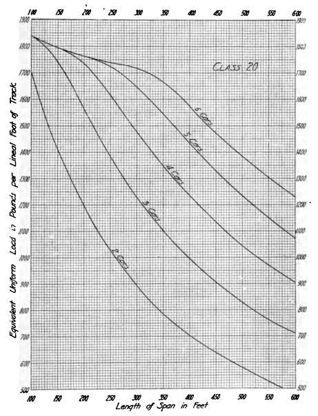
Fig. 6j. Equivalent Uniform Live Loads for Truss Spans with Class 20 Electric Railway Loading.
