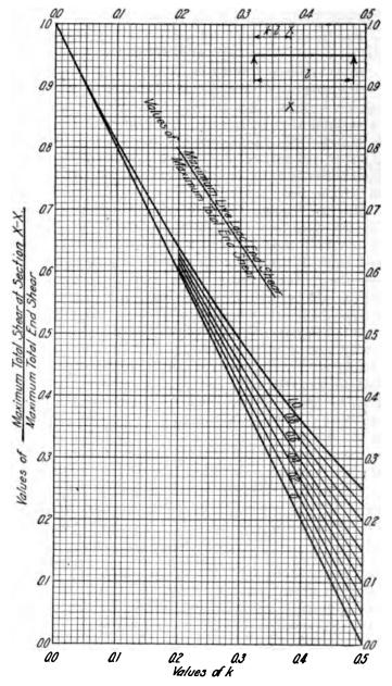
Fig. 21a. Total Shears throughout Plate-girder Spans Carrying Uniformly Distributed Live and Dead Loads.
