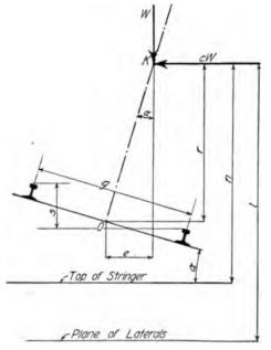
Fig. 8d. Forces Acting on a Structure on a Curve.
