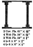
Fig. 22ddd. Proposed Top Chord Section for the 423-foot Spans of the Fratt Bridge over the Missouri River at Kansas City, Mo.
