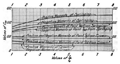
Fig. 37ee. Values of Live-Load Moment Coefficient Cm.
