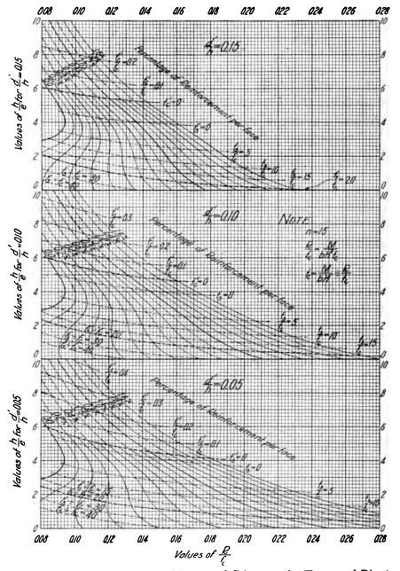
Fig. 37q. Diagram for the Design of Beams and Columns under Flexure and Direct Stress, with Reinforcement in Both Faces—for  $\frac{e}{h} > \frac{1}{7}$ .
