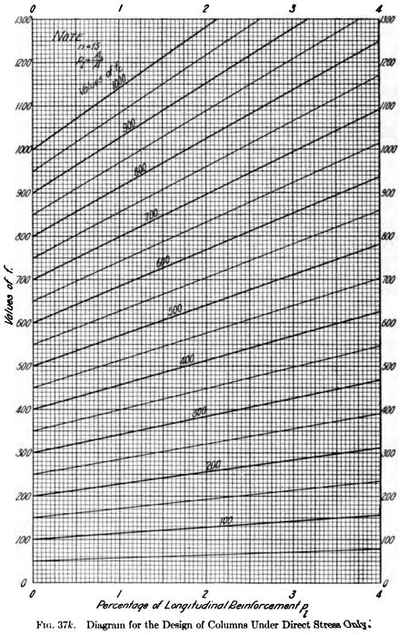
hand portion of Fig. 37j with p = 0.65% and  $\beta' = 30^{\circ}$ , trace horizontally to the line  $\beta = 0$ , and then vertically downward to R = 78, given in this case by the horizontal lines. We then read  $f_c = 520$  and  $f_s = 15,600$ .
