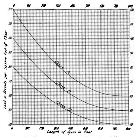
Fig. 60. Uniformly Distributed Live Loads for Highway Bridges.
