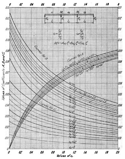
Fig. 37v. Moment Coefficients for Continuous Beams.
