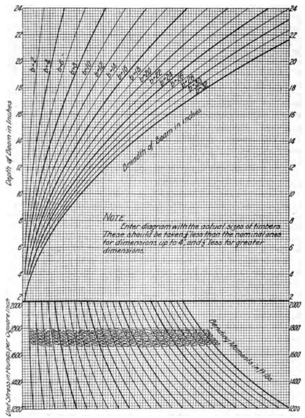
Fig. 16h. Diagram for Designing Timber Beams.
