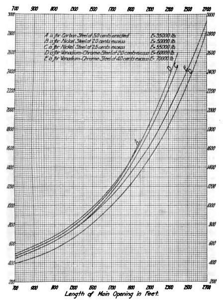
g. 4q. Comparative Costs of Double-track, Cantilever, Railway Bridges of Carbon teel and Mixed Alloy and Carbon Steels, Contrasting Vanadium and Nickel Steels.
