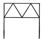
Fig. 20a. Outline of Sway Bracing Frame for Through Bridges with Parallel Chords.
