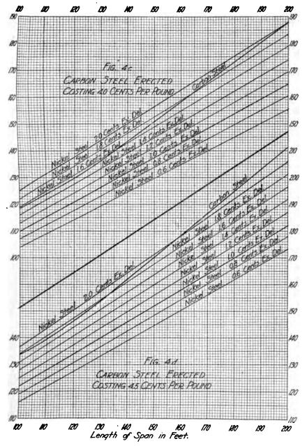
4c and 4d. Comparative Costs of Double-track, Through, Riveted, Pratt-truss Spans of Carbon Steel and Mixed Nickel and Carbon Steels.
