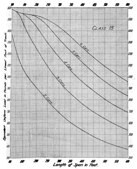
Fig. 6i. Equivalent Uniform Live Loads for Truss Spans with Class 15 Electric Railway Loading.
