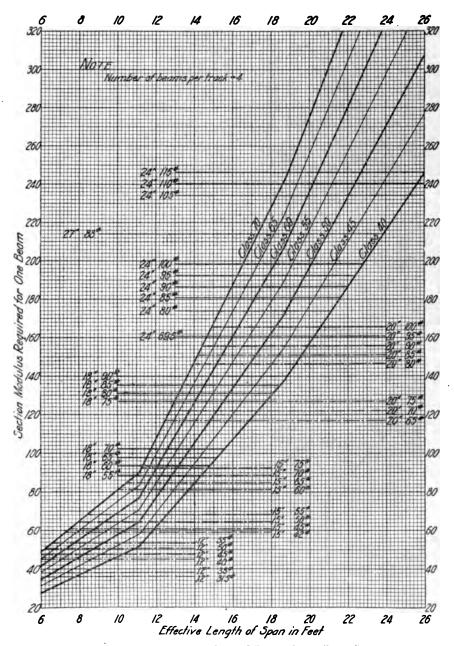
Fig. 21s. Diagram for Design of I-Beams for Railway Spans.
