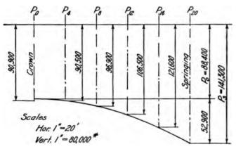
Fig. 37ii. Plot of Loads on Arch Rib.
