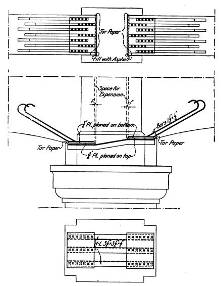
Fig. 37uu. Expansion Plates for Main Girders.
