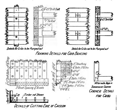
Fig. 41a. Details of Cutting Edge and Framing of Crib for a Pneumatic Pier.
