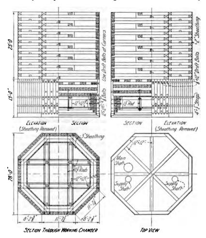
\*G. 41d. Details of Pneumatic Caisson for Pivot-pier of the Granville Street Bridge over False Creek in Vancouver, B. C.
