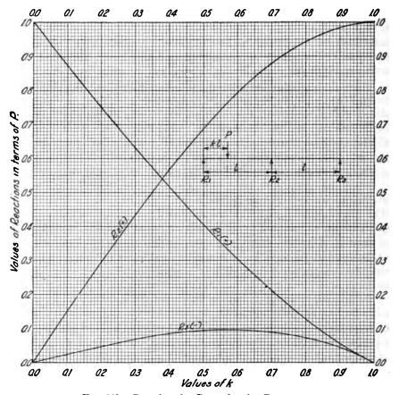
Fig. 29b. Reactions for Centre-bearing Draw-spans.
