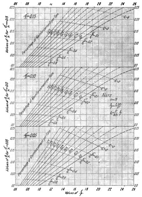
Fig. 37o. Diagram for the Design of Beams and Columns Under Flexure and Direct Stress, with Reinforcement in Both Faces—for  $\frac{e}{h} < \frac{1}{4}$ .
