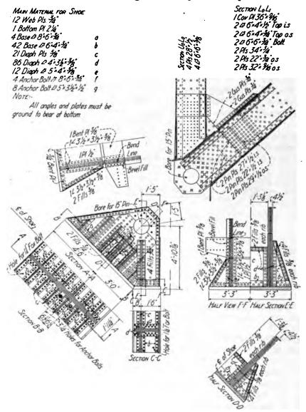
Fig. 26o. Pedestal Hinge for the Arch Span of the Canadian Northern Pacific Railway
