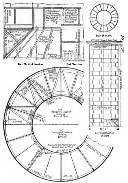
Fig. 40d. Open-dredging Caisson for the East Omaha Bridge over the Missouri River.
