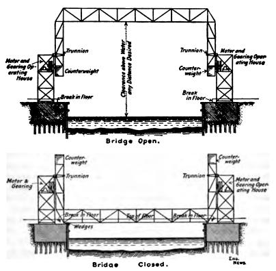
Fig. 28b. The Gyratory Lift Bridge.
