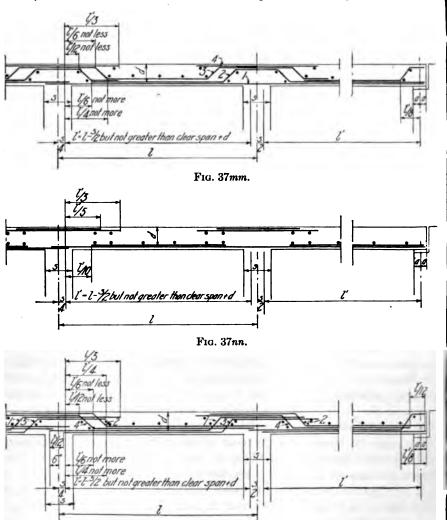
Fig. 3700. Arrangements of Slab Reinforcement.
