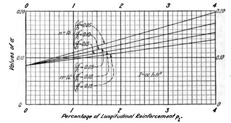
Fig. 37t. Moments of Inertia of Columns and Arch Ribs.
