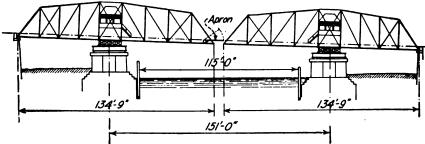
Fig. 28a. Double, Rotating, Cantilever Draw Bridge over the Cuyahoga River at Cleveland, Ohio.
