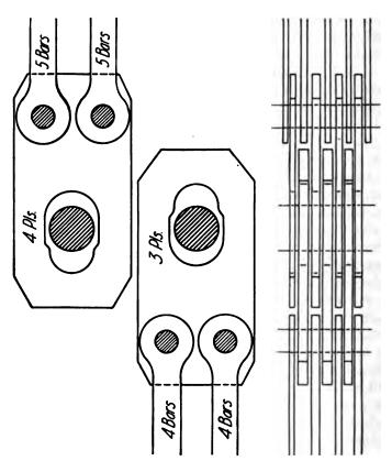
Fig. 25gg. Detail of Connection between Suspended Span and Cantilever Arm for Quick Erection.
