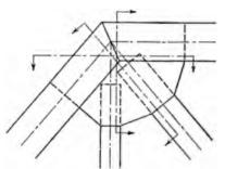
Fig. 22mmm. Sections for Testing Gusset-Plates at the Hip Joint.
