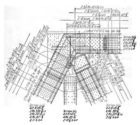
Fig. 22000. Hip Joint of the 287-foot Span of the O.-W. R. R. & N. Company's Bridge over the Willamette River at Portland, Ore.
