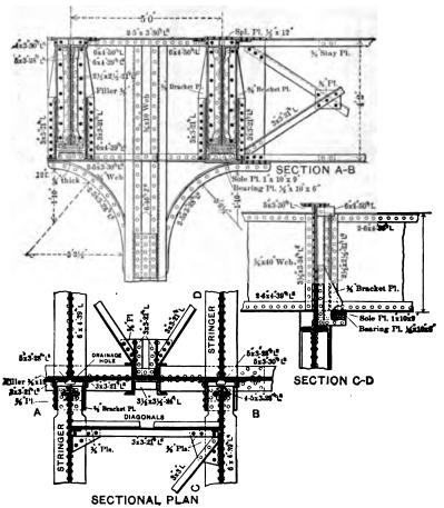
Fig. 24f. Details at Upper Part of Column with Expansion Girders for Elevated Railroads.
