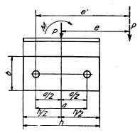
Fig. 16i. Layout of Base-Plate and Anchor Bolts.
