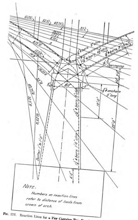
Reaction Lines for a Pier Carrying Two Equal Arch Spans.
