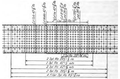
Fig. 22iii. Bottom Chord Tension Lap-splice for the 287-foot Span of the O.- W. R. R.
