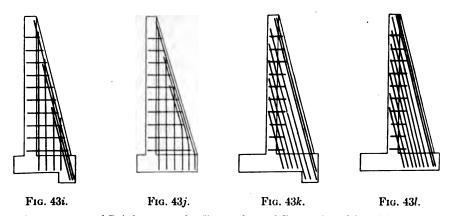
Arrangements of Reinforcement for Counterforts of Counterforted Retaining Wall.
