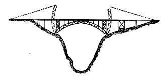
Fig. 26c. Three-hinged, Braced-rib Arch with Parallel Chords.
