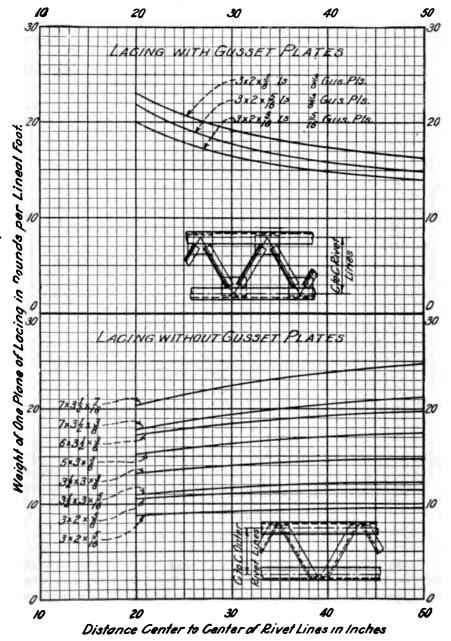
Fig. 16b. Weights of Angle Lacing.
