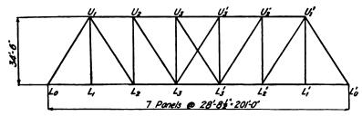
Fig. 11c. Truss Diagram of a 201-foot, Single-track-railway, Through, Riveted, Pratt-truss Span.
