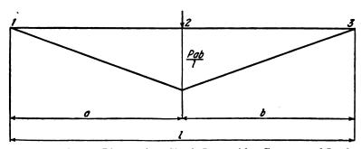
Fig. 12c. Moment Diagram for a Simple Beam with a Concentrated Load.
