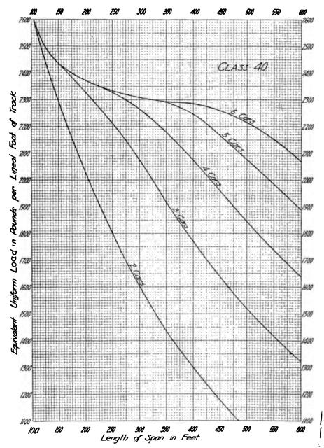
Fig. 6n. Equivalent Uniform Live Loads for Truss Spans with Class 40 Electric Railway Loading.
