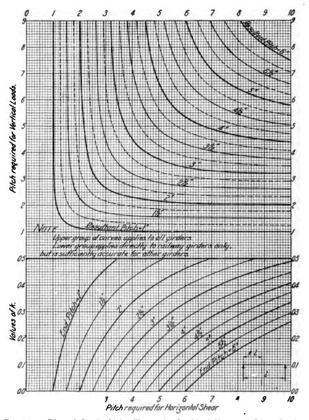
Fig. 21m. Rivet-pitches in Girder Flanges for Combined Shear and Direct Loads.
