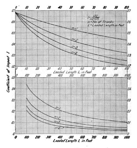
Fig. 7d. Coefficients of Impact for Electric Railway Bridges.
