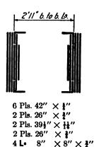
Fig. 22ccc. Typical Bottom Chord Section for the 287-foot Span of the O.-W.
