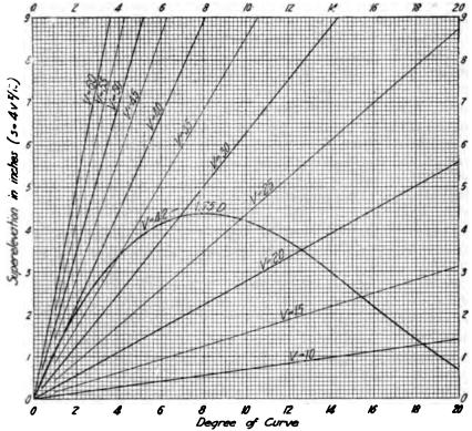
Fig. 8a. Superelevation for Tracks on Curves.
