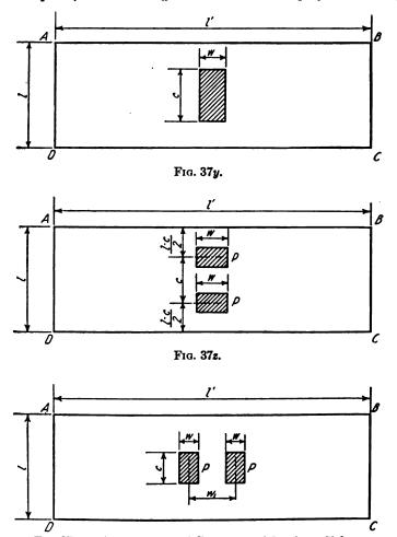
Fig. 37aa. Arrangements of Concentrated Loads on Slabs.
