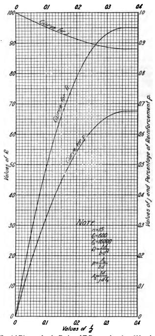
Fig. 37h'. Special Diagram for the Design of T-Beams when  $f_c=600$  and  $f_s=16,000$ .
