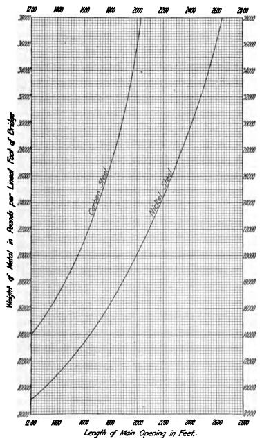
Fig. 4g. Probable Weights of Very-long-span Cantilever Bridges of Carbon Steel and of Nickel Steel.
