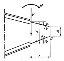
Fig. 211. Girder with Inclined Flanges.
