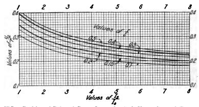
Fig. 37ff. Position of Point of Contraflexure for Arch Shortening and Temperature Stresses.
